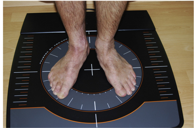
Fig 1. Baropodometric data collection in a patient with stroke: standing barefoot in a comfortable bipedal position on the platform with both heels separated 2 cm with forefoot creating a 30° angle.
